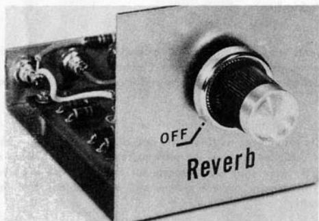
Hi-Fi, Stereo, or even added to your musical instrument amplifier. It uses the "Gibbs" (Hammond Organ) type IV spring delay, and is the same type used in the highest priced existing systems and is placed between the preamp and power amp, giving you that full music-hall sound. For more details on reverb springs send for specification sheets.
