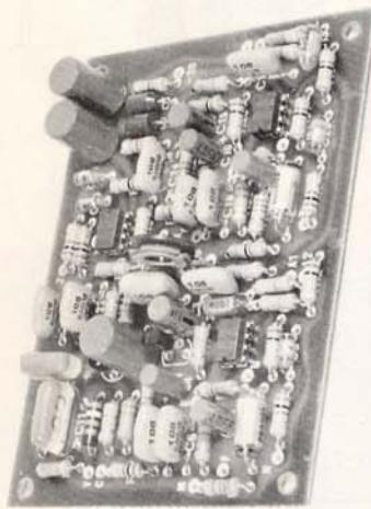
One straight preamp with only tone controls, one preamp with tremolo and reverb. All on one  $3\frac{1}{4} \times 4\frac{1}{2}$  circuit board. New op-amp circuit provides all these features and less than 0.1% distortion at 1.0 Volt output. Combine with one of our "Tiger" series, or 540 amplifiers for a complete system.
